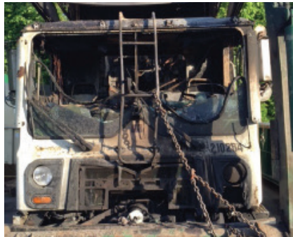
Example of a fire caused by hazardous materials thrown in the trash.
