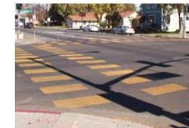
Multiple large parallel line markings are used to increase visibility where moderate to heavy pedestrian volumes exist and at mid-block crossings or where pedestrians are not expected.
